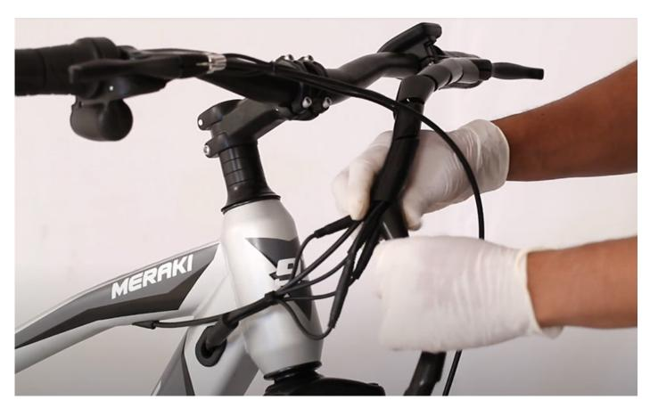
STEP 13: Wrap the spiral harness around the cable
