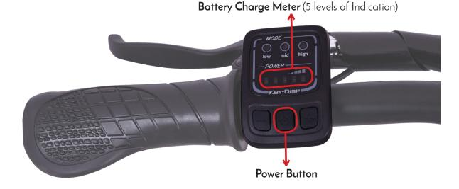
Once the E-Bike and Monitor display are ON, verify that the Battery Charge Meter (LED display) shows sufficient charge for your ride. If the battery does not have sufficient charge for your ride, please refer to instructions on how to charge the Battery.
