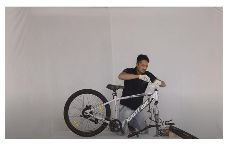
STEP 5-6: Remove the cable ties, foam and detach the front wheel and handle bar from the frame
